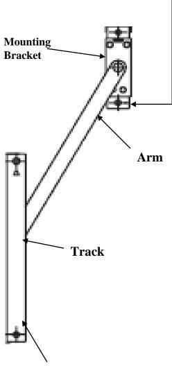
The track is attached to the sash flush with the bottom outside edge.
